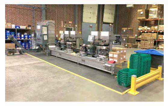
Our new kitting machine makes bagging and kitting a much more automated process, increasing efficiency and productivity.
